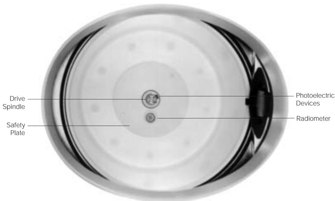
Figure 1-2. The Rotor Chamber
