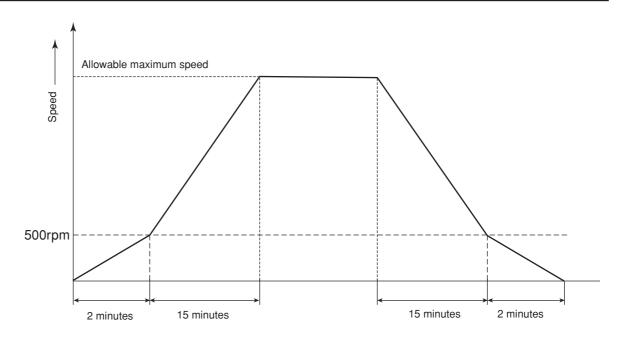
Fig. 2-4-1 Operation with setting ACCEL = 0 and DECEL = 0
