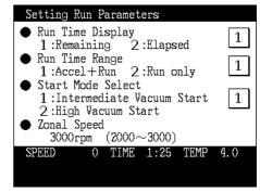
Fig. 2-8-11 Run condition setting screen
