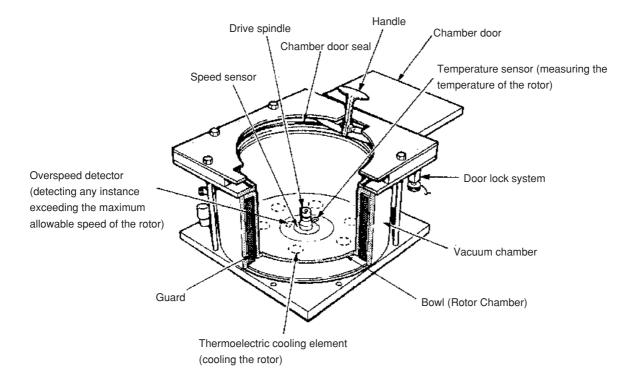
Fig. 1-2-3 Rotor chamber
