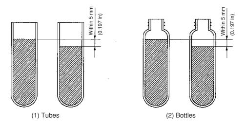
Fig. 2-1-2 Balancing tubes/bottles containing a sample solution
