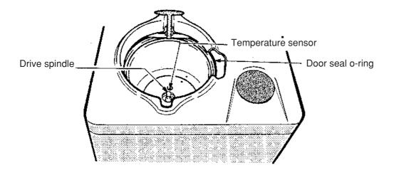
Fig. 3-1 Rotor chamber
