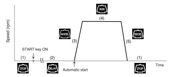
Fig. 2-5-6 Run mode display (RTC)
