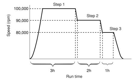
Fig. 2-5-4 A typical step-mode run
