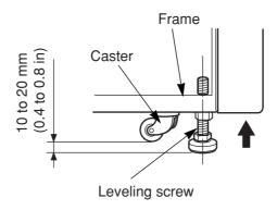
Fig. 5-2 Leveling Adjustment
