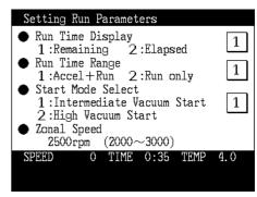
Fig. 2-8-8 Run condition setting screen
