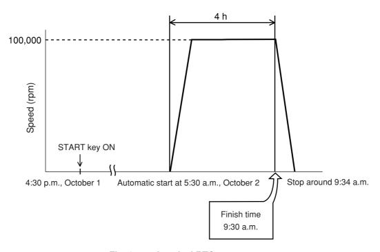
Fig. 2-5-5 A typical RTC run
