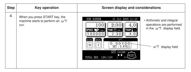
NOTE When the  $\omega^2T$  display field reaches the set value of  $\omega^2T$ , the machine decelerates and stops. During deceleration, the  $\omega^2T$  display field continues to accumulate value until the rotor stops and the run ends.
