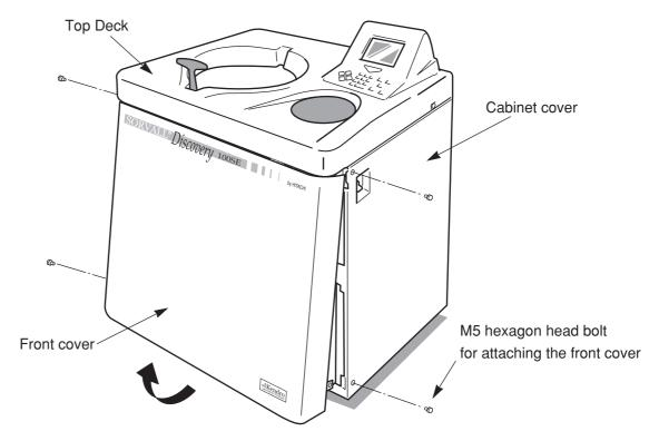
Fig. 2-7-1. Removing the front cover
