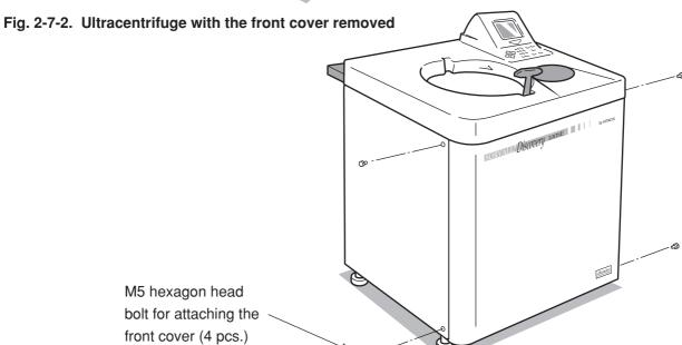
Fig. 2-7-3. Installing the front cover
