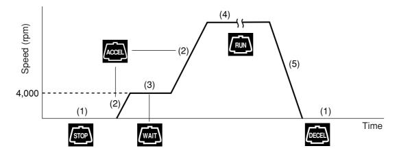
Fig. 2-3-3 Displays of run modes
