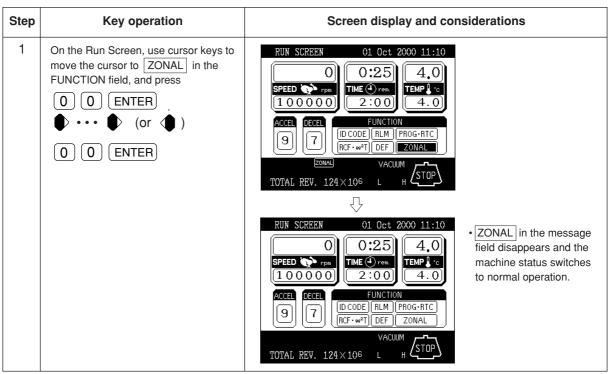
NOTE If no key operation is performed for 30 seconds, the cursor disappears and any entry is disabled. At that time, press the cursor key to cause the cursor to blink once again.
