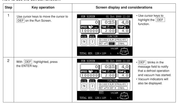
Defrost operation will heat the evaporator gradually and after the lapse of 10 minutes, the defrost operation and vacuum ends automatically.
