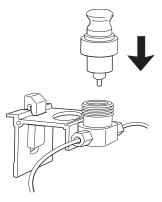
**Electrode regeneration:** If the electrode has dried out, immerse the lower end of the electrode in buffer with a 1:1 mixture of pH 4 buffer and 1 M KNO<sub>3</sub> overnight.
