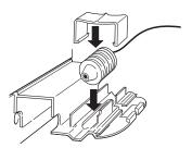
2 Connect the conductivity cell to the socket Conductivity Flow Cell on the rear panel of the instrument.
