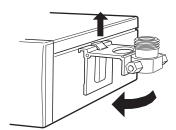
If the flow cell holder is not used, the flow cell must still be installed at an angle of 30° from the vertical with the outlet placed higher than the inlet to prevent air bubbles being trapped in the cell.
