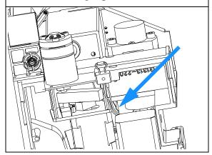
**3** Connect the connector to the connector (labelled "leak sensor").
