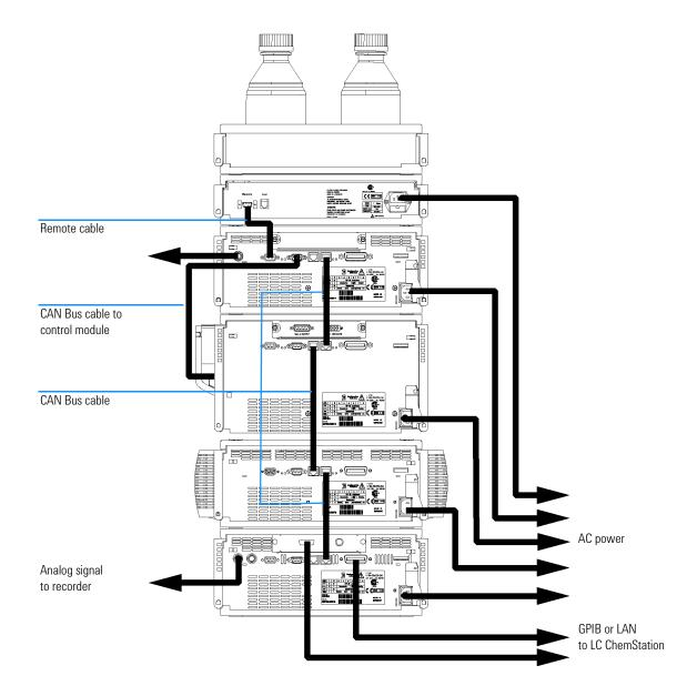
Figure 3 Recommended Stack Configuration for a Thermostatted ALS (Front View)
