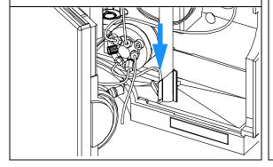
**7** Place the stator face in place on the stator head.
