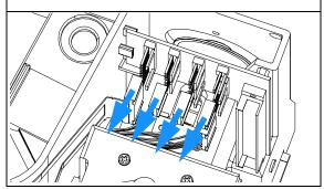
**2** Remove the two fixing screws, and lift out the board.
