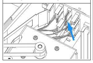
16Remove the metering head assembly (see "Gripper Arm" on page 123).
