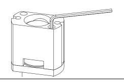
**5** Use a small screwdriver to carefully remove the seal. Clean the chamber with lint-free cloth. Ensure all particular matter is removed.
