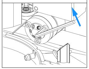
**3** Remove the stator head and stator face.
