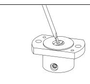
7 Place the piston guide on top of the seal.
