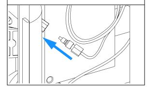
**7** Use "Needle Up" to lift the needle to a position approximately 2mm above the seat.
