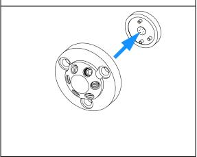
4 Place the stator face in place on the stator head. Ensure the pins on the stator engage in the holes in the stator head.
