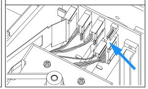
**2** Feed the cable of the new sensor through the base of the sampling unit to the SUD board.
