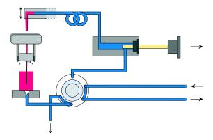
When the metering unit has drawn the required volume of sample into the sample loop, the needle is raised, and the vial is replaced in the sample tray. The needle is lowered into the needle seat, and the injection valve switches back to the mainpass position, flushing the sample onto the column (Figure 34).
