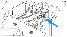
**6** Fix the valve assembly in place securely with the three screws.
