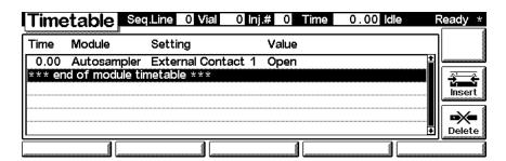
Press the F7 key (**Insert**) to add timetable events. Use the F6 key (**Done**) to view the entered lines of the timetable.
