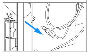
Loosen the fixing screw, and lift out the needle.
