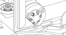
**2** Loosen each fixing bolt two turns at a time. Remove the bolts from the head.
