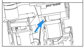
**5** Connect the valve cable to the connector (labelled "Valve Assy").
