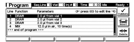
Press the F7 key (**Insert**) to add program events. Use the F6 key (**Done**) to view the entered lines of the timetable.
