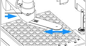
**4** Hold the paper clip in place, press the gripper release button and rotate the gripper arm to the right.
