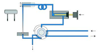
Next, the needle is raised, and the vial is positioned below the needle. The needle moves down into the vial, and the metering unit draws the sample into the sample loop (Figure 33).
