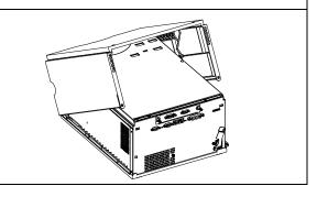
**5** Unscrew the three screws on the top plate. Remove the top plate.
