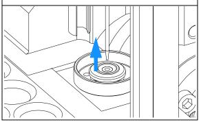
**8** Ensure the needle is aligned with the seat. If required, bend the needle slightly until the needle is aligned correctly.
