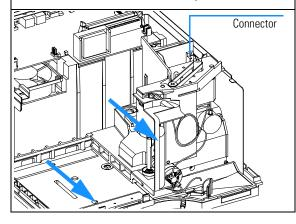
**6** Install the pump and column thermostat capillaries (ports 1 and 6) in the injection valve.
