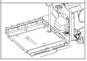
**7** Slide the tray base back to disengage the tray base from the sampling unit.
