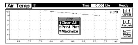
Press F6 key (**Select**). Here you can add additional on-line signals (maximum are 3). Additional signals could be also pressure or temperature signals from other modules. Use the Right/Left arrows to switch between Available and Selected Signals. Use the F8 key (**Move**) to enter available signals into the box for selected signals or vice versa.
