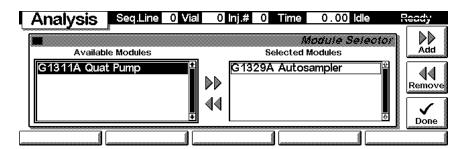
Here, e.g. the quaternary pump parameters are shown on the display as well. The number of parameters on the display are restricted as additional modules are added. A maximum of 4 modules are shown automatically. If more modules are in the system, you have to chose in Setup view. The number of parameters on the display are restricted as additional modules are added.
