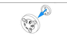
**5** Install stator head and stator face. Tighten the bolts alternately two turns at a time until the stator head is secure.
