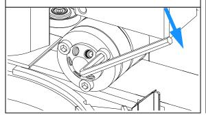
10 Slide the waste tube into the waste holder in the leak tray.
