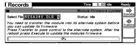
Use the Esc key to receive **Views** on the F5 key. Choose **System** from the pull-down menu. Use the F3 key (**Records**) to select the ALS. Use the F5 key (**FW Update**) to enter the Update section. Select the a file from the PCMCIA card (1313nnnn.DLB or 1329nnnn.DLB) and press execute. When the update has finished the update, press F7 key (**Transfer**) to return the module into the normal mode (LED on module should stays yellow).
