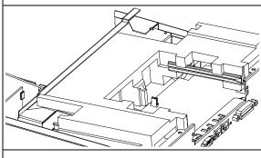
**3** Fix the top plate in place with the three screws.
