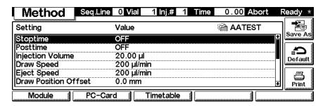
Use F2 key (**PC-Card**) to save a method on a PCMCIA card. Use the Right/Left arrows to switch between PC-Card and Instrument window. Use the UP/Down arrows to select the method. Use the F7/F8 keys (**Copy**) to enter available signals into the box for selected signals or vice versa. Press the **m**-key to open the context sensitive menu.
