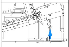
**5** Lift the sampling unit and tray base out of the autosampler.
