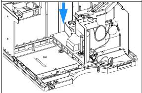
**5** Slide the sampling unit and tray base forwards. Ensure the sampling unit connector is seated correctly.
