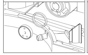
**3** Remove the stator head, stator face and stator ring.
