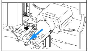
4 Disassemble the metering head assembly.
