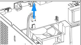
2 Lift the fan, and carefully pull the fan out of the foam.
