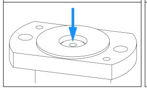
**3** Remove the two fixing bolts from the base of the metering head assembly.
