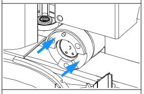
**8** Install stator head and stator face. Tighten the bolts alternately two turns at a time until the stator head is secure.
