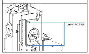
**3** Install the new board. Ensure the board is positioned between the board guide.
