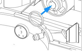
**6** Install the stator ring. Ensure the housing is flush against the valve body.
