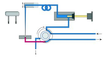
When the sample sequence begins, the valve unit switches to the bypass position (Figure 32). Solvent from the pump enters the valve unit at port 1, and flows directly to the column through port 6.
