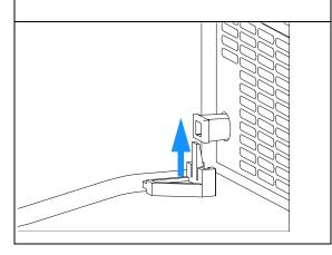
Install the bottom foam. Ensure the cables are positioned as shown.
