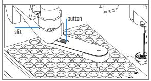
**2** Rotate the arm approximately 2.5cm (1 inch) to the left and insert the straightened paper clip into the slit.
