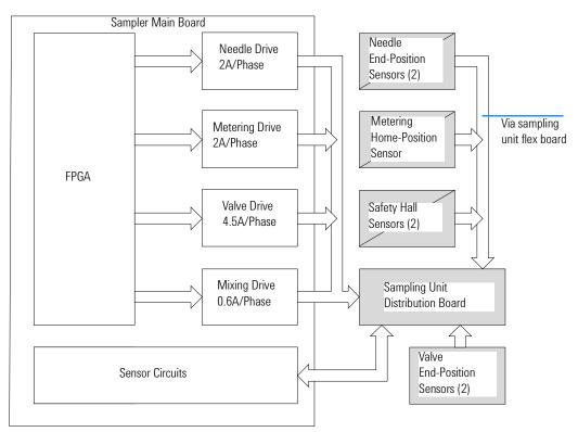
Figure 40 Autosampler block diagram
