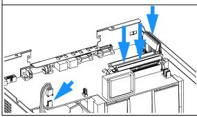
6 Replace GPIB and RS232 connector screws.
