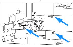
${f 3}$  Remove the injection-valve assembly.
