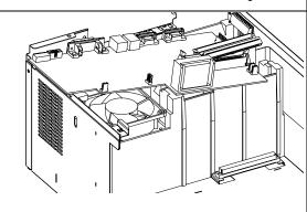
4 Install new board. Ensure ribbon cables are positioned in the slot in the board.
