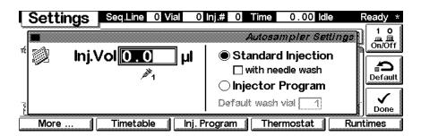
Use the **m**-key for the context sensitive menu. The **Status** command pulls up a monitor screen displaying details of injections and the sample tray. **Reset** will initialize the autosampler.
