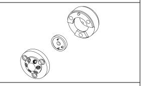
**5** Install the new rotor seal and isolation seal (if required). Ensure the metal spring inside the isolation seal faces towards the valve body.
