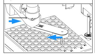
**3** Rotate the gripper arm slowly from left to right and apply a gentle pressure to the paper clip. The clip will engage on an internal catch and the rotation of the arm will be blocked.
