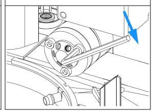
**6** Reconnect the pump capillaries to the valve ports (see "Hydraulic Connections" on page 31).
