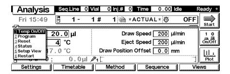
In the Setup view, e.g. the quaternary pump can be added to the view.
