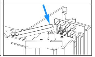
**21** Install the metering-head assembly (see "Gripper Arm" on page 123).
