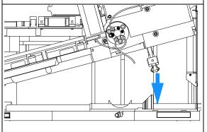
**4** Place the sampling unit and tray base into the autosampler.
