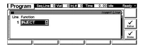
Use the m-key for the context sensitive menu. It gives you additional tools for the timetable. The F8 key (Validate) will check the injector program for errors.
