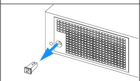
**6** Insert the coupler onto the switch of the new power supply.
