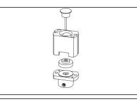
**6** Install the new seal. Press the seal firmly into position.
