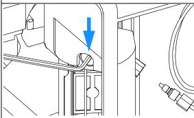
Select "Needle Down". Repeat the selection until the needle arm reaches its lowest position.
