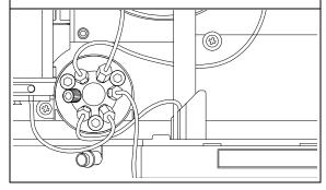
**7** Slide the waste tube into the waste holder in the leak tray.
