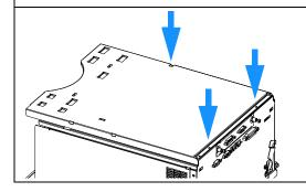
**2** Engage the slot on the top plate onto the side plate.
