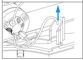
**3** Slide the sampling unit and tray base back to disengage the sampling-unit connector.
