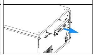
${\bf 3}$  Move the safety lever to the left. Lift the clips on the top cover.
