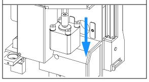
**18** Feed the motor cable through to the SUD board. Connect the cable to the connector, labelled "Needle M".
