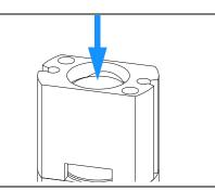
11 Install the metering head assembly in the autosampler. Ensure the large hole in the metering head is facing downwards.
