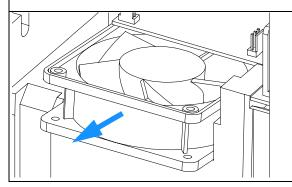
**3** Install the new fan. Ensure the cable is installed as shown.
