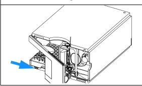
**2** If installed, remove the ECB board.
