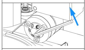
$\begin{tabular}{ll} {\bf 4} \ Remove \ the \ rotor \ seal \ (and \ isolation \ seal \ if \\ required) \end{tabular}$
