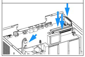
3 Slide ASM board out of the autosampler.
