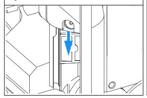
Insert the new needle. Align the needle in the seat, then tighten the screw firmly.
