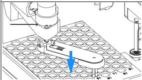
**6** Replace the gripper arm by holding the paper clip in place, pushing the gripper arm into the holder and rotating the gripper arm to the left.
