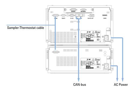
Figure 15 Connection at the rear of thermostatted Autosampler
