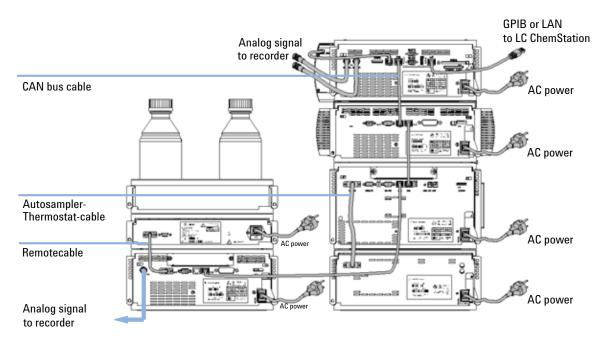
Figure 11 Recommended Stack Configuration - Thermostatted Autosampler (Rear View)
