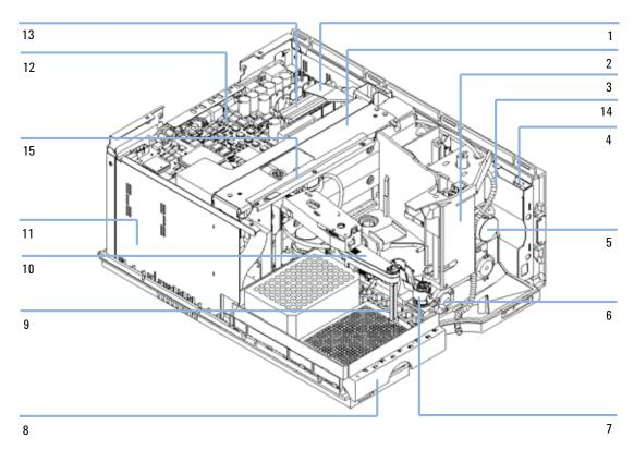
Figure 24 Autosampler Main Assemblies
