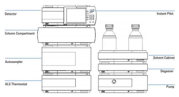
Figure 10 Recommended Stack Configuration - Thermostatted Autosampler (Front View)
