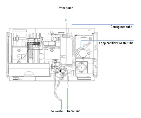
Figure 16 Hydraulic Connections
