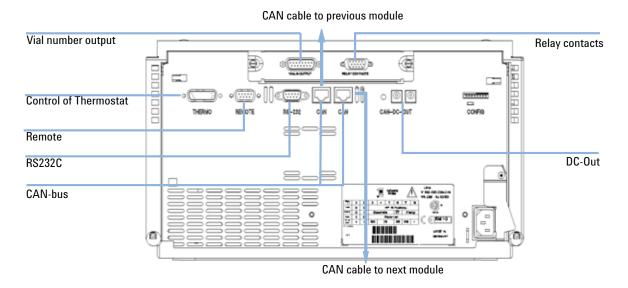
Figure 12 Cable Connections
