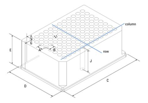
Figure 19 Well Plate Dimensions (straight)
