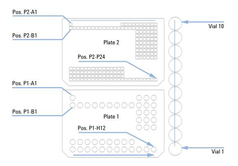
Figure 18 Numbering of vial and well plate position
