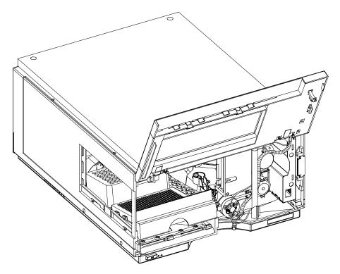
Figure 17 Installing the Sample Tray
