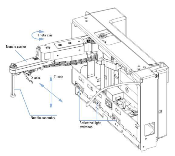
Figure 6 Needle/Sample Transport Assembly
