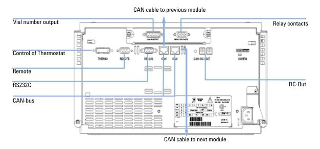
Figure 7 Autosampler Electrical Connections
