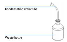
Figure 13 Condensation leak outlet
