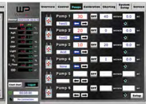
Pumps Control speed, direction, total volume and flow rate
