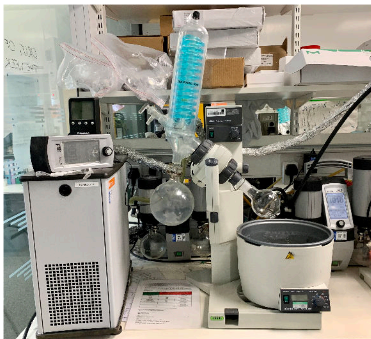
Figure 1. Existing rotovap set up used at the University of Oxford, tested during the case study.
