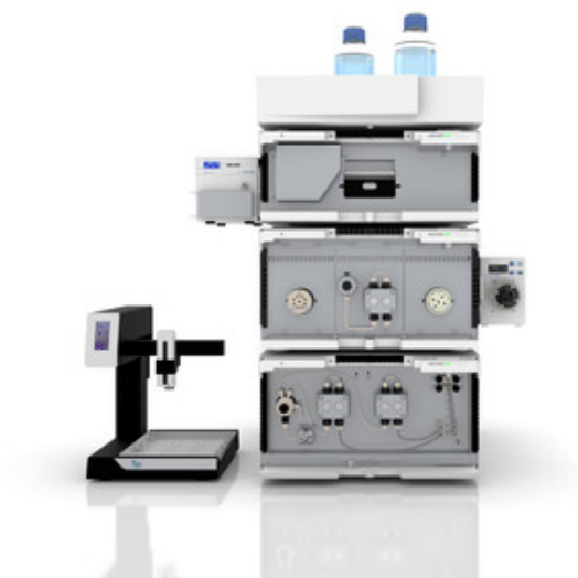
AZURA Bio Lab System Advanced: exemplary configuration for automated two step applications including the optional fractionation valve
